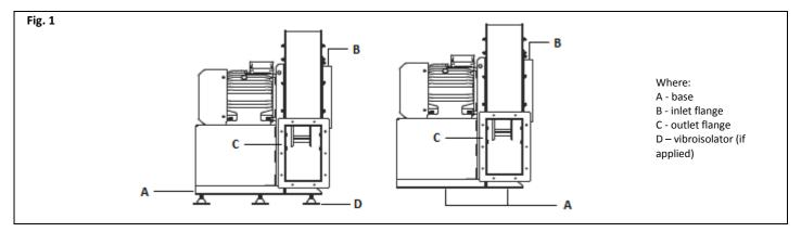
•Supporting construction has to be solid enough in order to carry the weight of the fan and generated vibration (including fan damage). The fan cannot be exposed to vibration.
